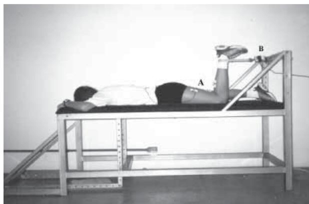
**Figure 1.** Position of the subject in the isometric test. A. Placement electrode. B. Load cell.
