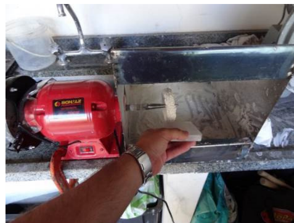
Figure 5. Piece receiving polishing with brush and Pumice stone.
