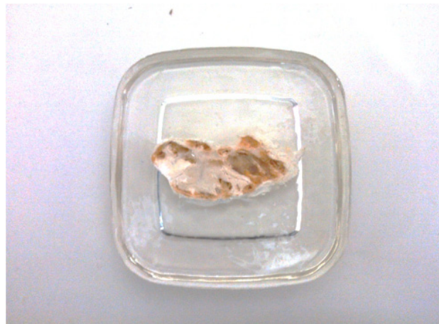
Figure 10. Part degraded due to the lack of resin.
